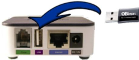
**Step 2\*:** From a WiFi enabled device, e.g. computer, tablet or smart phone, open its network settings and connect to a WiFi network called “**OBiWiFi\_Setup**.” Your browser-equipped device will automatically connect to the OBiWiFi\_Setup network.
